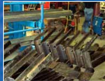
*Fabrication of custom fitted cornice supports. All work completed at Design Installation Systems' shop.*
